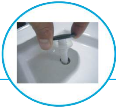
Insert water sprayer "R" and silicone washer on top of slide. Hand tighten the retainer nut beneath the slide.
