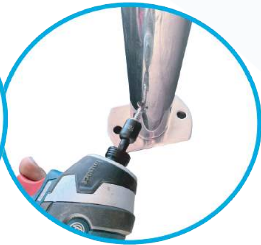
Install screws "Q" using the 10mm nut tip "DD"
